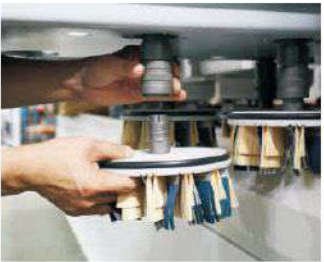
Fast connector design to ensure fast change
