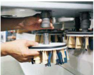
Fast connector design to ensure fast change
