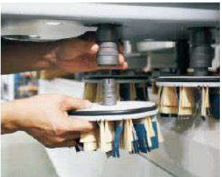
Fast connector design to ensure fast change
