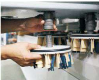
Fast connector design to ensure fast change
