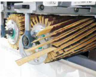
Replace the abrasive material directly
